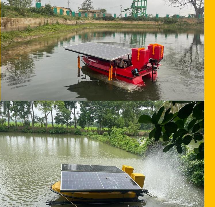
Integrated solar power operated floating device that provides the right ecosystem for proper growth of Fish & Prawn stocks.
