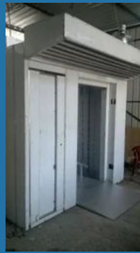
Rotary Rack Oven
