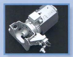
▶ Elimination of the clutch brake, simplified mechanics, and outstanding reliability are the main characteristics of the Direct Drive motor, which has always been fitted to Panter machines. Ready response guarantees high quality fabrics, beating overload peaks and bringing down energy consumption.
