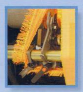
► A comprehensive range of electronically controlled devices, such as lateral and central scissors, independent selvedge formation devices, mean setup and changing style is easy and cost-effective.
