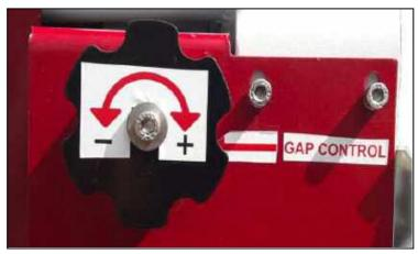
should be adjusted using the feeler gauge (0.3-0.5 for small grain rice and 0.5-0.8 for medium and long grain rice).
